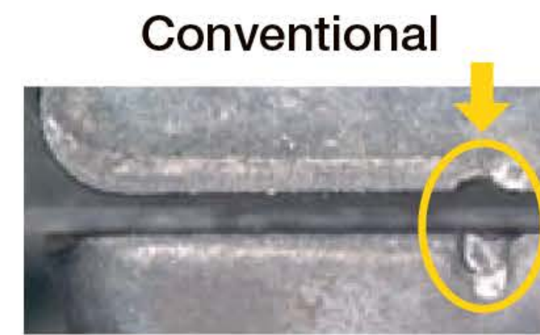
Edge fracture occurred due to low cutting edge strength
